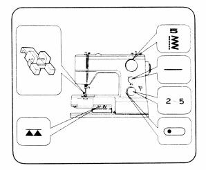
Position a button and material under foot. When needle comes to left side of stitch, lower foot. Raise needle and adjust zigzag width so that needle comes to right hole of button.
